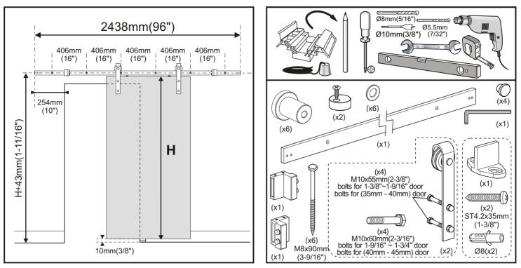
To obtain the maximum weight capacity, all rail mounting fasteners must be mounted directly into solid wood. Do NOT install directly onto a drywall surface. A solid wood header is recommended as shown in instruction box 2.
