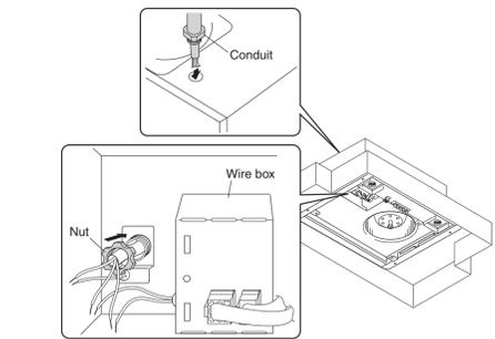
3 Connect the electrical wires as follows: Connect wires tightly and securely using wire connectors (not supplied).
