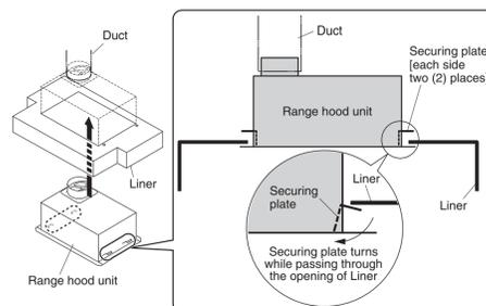
2 Align 4 screw holes of the liner and range hood unit, then fix securely using the supplied screws and nuts.
