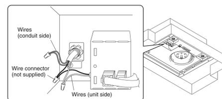
4 Replace the wire cover with the screw removed previously. Make sure that all wires are connected properly and enclosed inside of the wiring compartment.
