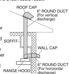
2 The range hood unit must be mounted to a liner which has the following dimensions. Install the liner securely after checking that the opening size of the liner is the same as the figure below.
