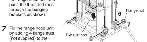
**Note:** Check that the range hood unit is fixed at the specified height horizontally and adjust if not.
