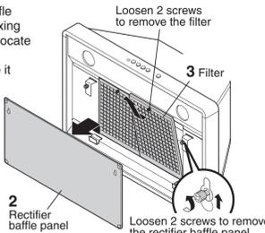
3 Detach the filters by turning the fixing knobs counter-clockwise, and disengaging them from the supporting groove.
