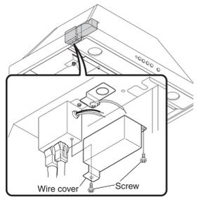
3 Connect the conduit through the connecting hole of the body using the nut previously removed.
