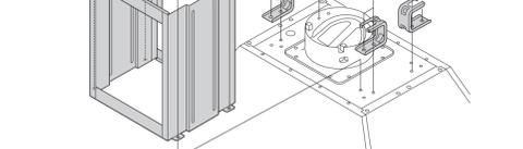
7 Fix the range hood unit by adding 4 flange nuts (not supplied) to the threaded rods as shown.
