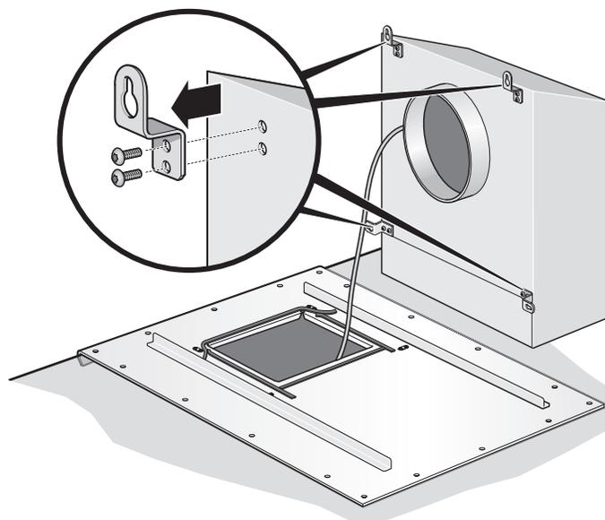
Mounting the blower on the roofplate
